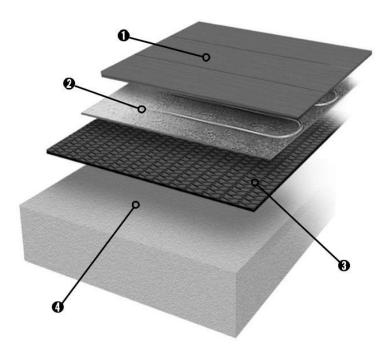
1. Hessian Backed Carpet with Underlay or Floating Wooden Floor. Maximum Carpet tog 1.7, Underlay tog 0.8. Ideal wood thickness up to 18mm
