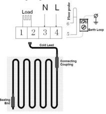
For the correct connection of the Rayomax mat, please, pay attention to the colours of the installation wires. The blue and brown installation wires are connected with the heating conductor and are to be connected to the thermostat. The earth wire must be connected to the earth.
