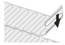
To allow continuous earth current, each time the mat is turned, you must use the aluminium strips provided to bridge the gap and cover the exposed cable. If there is no gap, you must still use the aluminium strip in case there is any future movement.
