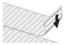
To allow continuous earth current, each time the mat is turned, you must use the aluminium strips provided to bridge the gap and cover the exposed cable. If there is no gap, you must still use the aluminium strip in case there is any future movement.
