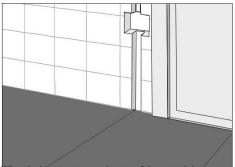
When laying carpet over the top of the mats it is advisable to lay a 6mm baton around the edges for the grippers
