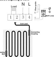
For the correct connection of the Rayoflex mat, please, pay attention to the colours of the installation wires. The blue and brown installation wires are connected with the heating conductor and are to be connected to the thermostat. The earth wire must be connected to the earth.
